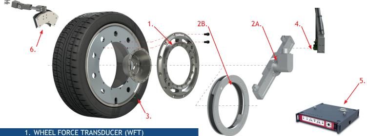
Measures: longitudinal (Fx), lateral (Fy), and vertical (Fz) forces, camber (Mx), torque (My), and steer (Mz) moments
